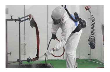
A painter should also only use nitrile gloves, which protect against isocyanate sensitization. A full mask is required, preferably with a fresh air supply, which also keeps the painter cooler. Booties are optional and can protect a painter's shoes from overspray.
