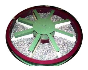
Rotating Carousel Divider Option allows parts to be finished without part to part contact. The number of removable dividers is determined by your production rate. Nylon dividers can be removed to adjust spacing for larger parts. Carousel rotates on the heavy duty center
