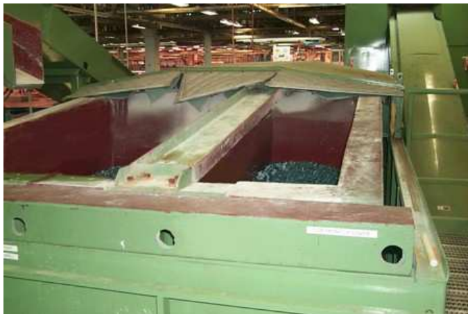
Photo to the left shows the OHD 9696 Tub with Removable Divider having the Media unloaded using the Automated Material Handling System. It consists of a Vibratory Screener for media sizing, Conveyor for transfer to a Storage Hopper, and a Return Conveyor back to the Vibratory Machine.
